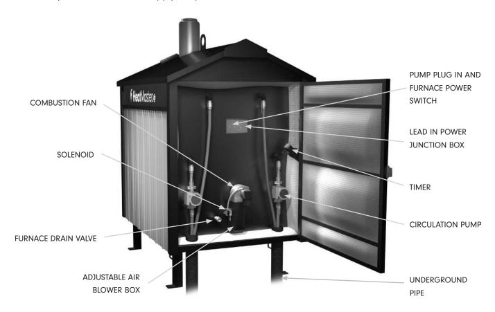
At least one pump must be circulating at all times or the water in the furnace may boil. A continuous pump is also useful for freeze protection in temperatures below 32°F.
