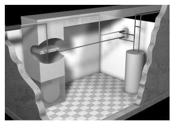
Forced air furnace with water-to-air exchanger
