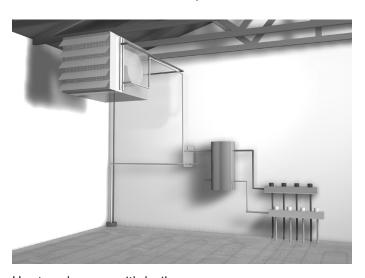
Heat exchanger with boiler
